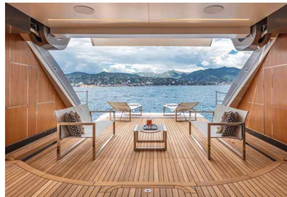
The huge beach club on Chorusline is an excellent space for lounging or entertaining. The transom opens vertically while panels on either side fold down and can be joined to the aft running board by detachable panels to become one continuous space, open on three sides to the air and views. The side panels double as doors to the garage for tender and jet ski
