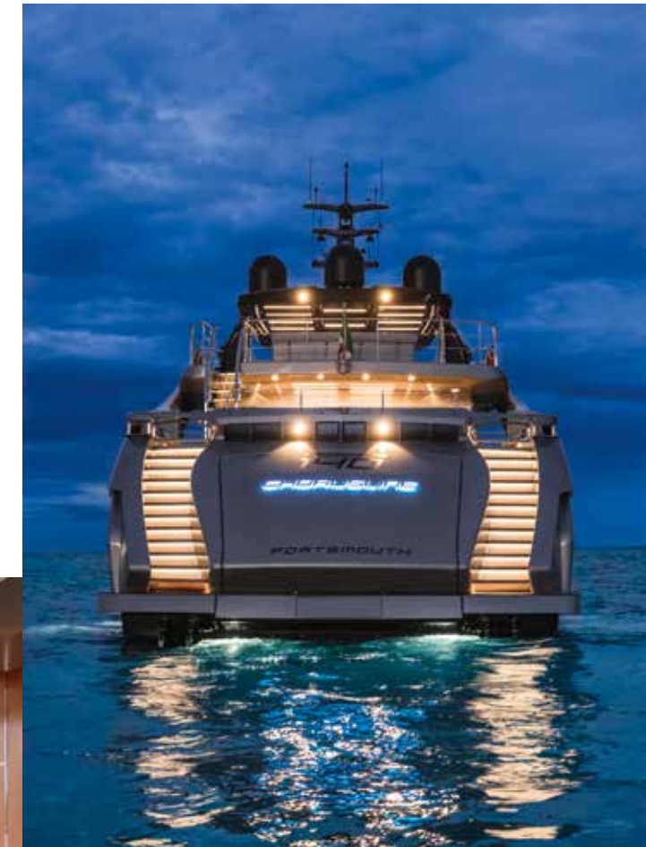
The huge beach club on Chorusline is an excellent space for lounging or entertaining. The transom opens vertically while panels on either side fold down and can be joined to the aft running board by detachable panels to become one continuous space, open on three sides to the air and views. The side panels double as doors to the garage for tender and jet ski
