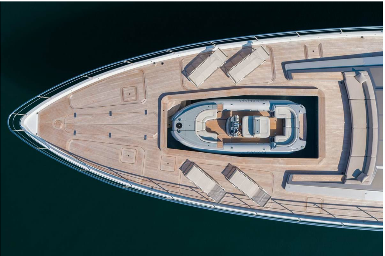
Forecastle deck pool and tender storage
